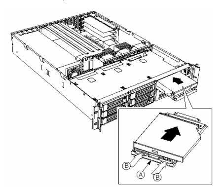
Figure 27: Installing a CDROM/FDD Module
